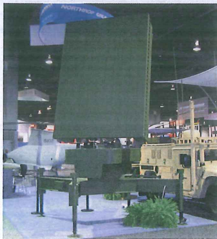
■ (Above) Mockup of Northrop Grumman's G/ATOR multirole radar, which was originally designed to be transported as a complete system by a single HMMWV.
