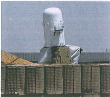
■ A Raytheon LPWS seen at Basra in mid-2008. WLRs integrated into a networked C-RAM system provide such base protection assets with early warning and trajectory information to achieve successful hard kills.
