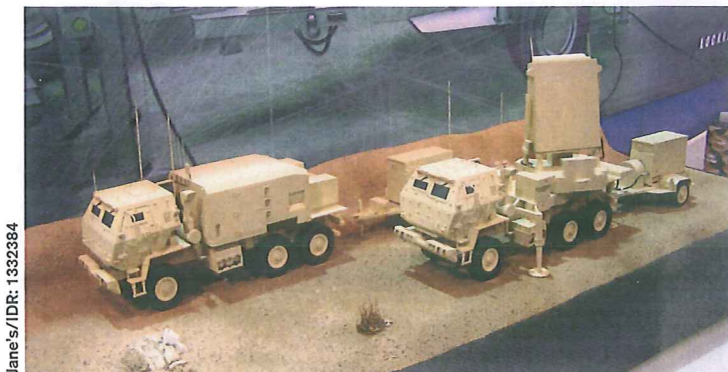
■ Model of the complete EQ-36 vehicle set, showing the antenna group on the vehicle to the right and the Burtel operations shelter on the other.
