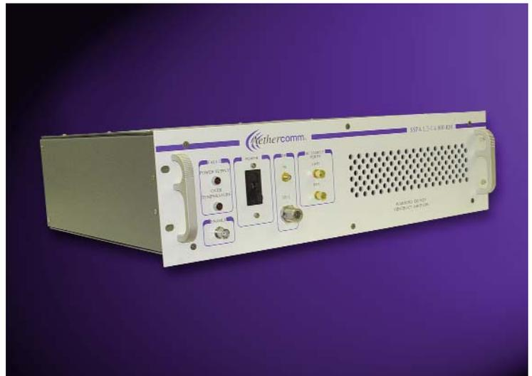
accessible via a BNC connector. There are RF sample ports for forward and reflected power via SMA female connectors. There is an over temperature alarm on the front panel of the rack mount assembly. The rack is fused for over current conditions with the fuses easily accessible. The PA is protected from an open or short-circuited placed on the output RF port of the unit.
