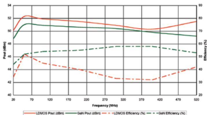
Figure 2: VHF/UHF amplifier LDMOS versus GaN comparison
