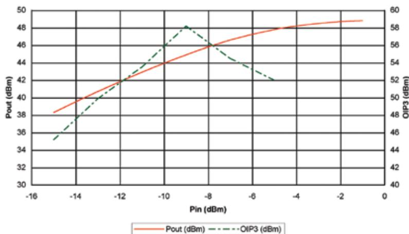
Figure 1: L-band amplifier output power versus OIP3
