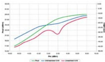
**Figure 2. RMPA29000 C/I3 Performance @ 25 ° C - LMDS Low End**
