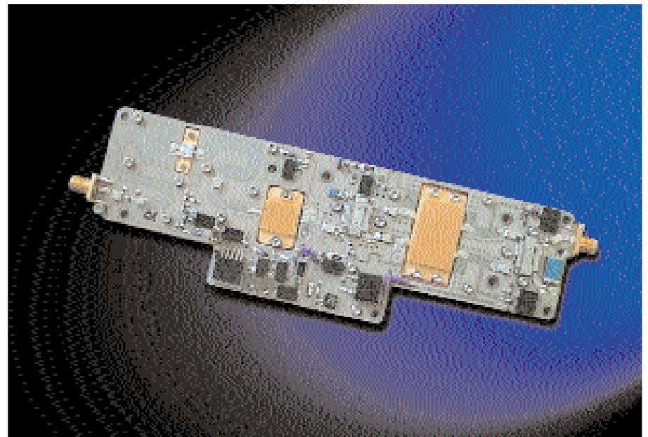
Aethercomm's 100 Watt S Band Solid State Power Amplifier
