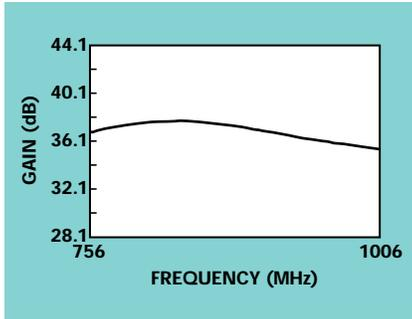
▲ Fig. 1 cellLNA2 maximum gain at 25°C.
