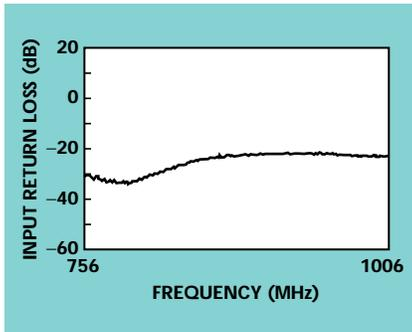
are shown in **Figures 1, 2** and **3**, respectively. These data show broadband performance from 756 to 1006 MHz. The gain response for this amplifier has been optimized for the 824 to 849 MHz AMPS system.
