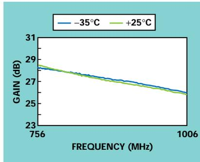
shows the amplifier's response from  $-35^\circ$  to  $+25^\circ\text{C}$ , indicating a gain variation of 0.15 dB. **Figure 5** shows the gain change from  $25^\circ$  to  $85^\circ\text{C}$ , where the gain variation over temperature is almost indistinguishable.
