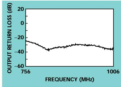
▲ Fig. 3 cellLNA2 output return loss at 25°C.
